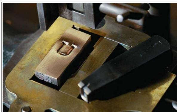
Fig.5: Poinçon et matrice.
